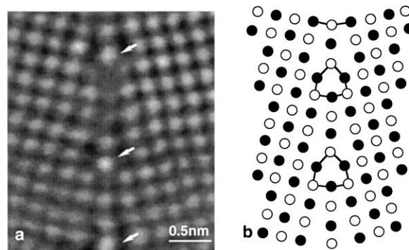
FIG. 1. (a) Z-contrast image of a symmetric 24° [001] tilt grain boundary in a MgO bicrystal. The white arrows highlight boundary columns with extra intensity. (b) Boundary structure model directly determined from the image. The open and closed circles indicate the location of the cations and anions on a single (001) plane.
