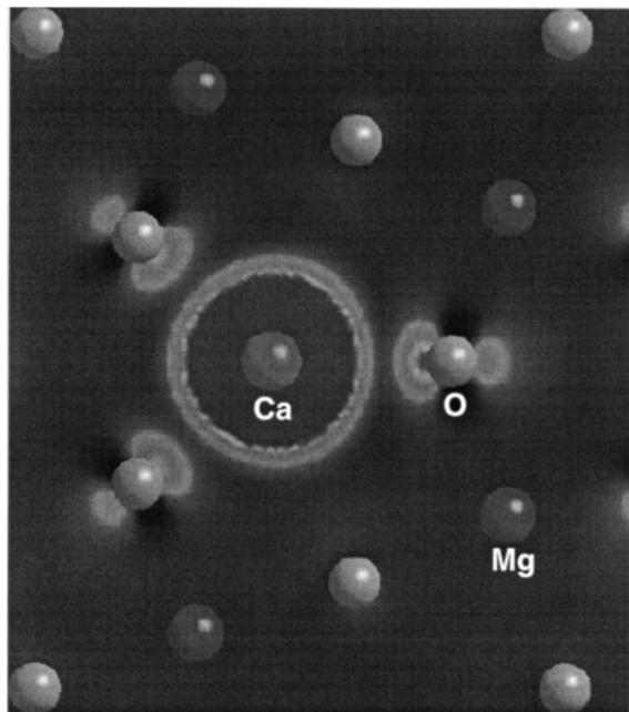
FIG. 4. Calculated charge density difference plot on a {001} plane perpendicular to the tilt axis showing the electron redistribution around the oxygen atom induced by the presence of Ca in the boundary.
