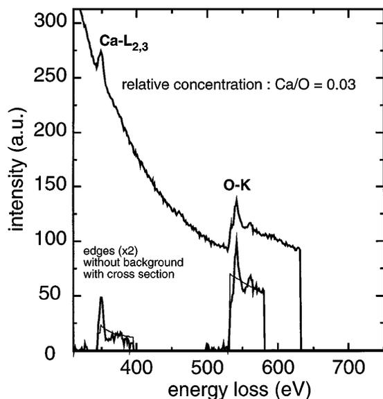
FIG. 2. EELS spectrum from an energy loss range containing both the oxygen  $K$  edge and the Ca  $L_{2,3}$  edges showing the presence of Ca in the grain boundary region. Calcium is not detected away from the boundary. Also included are spectra with the background subtracted that determine the relative concentration of Ca to O in the boundary region is 0.03.
