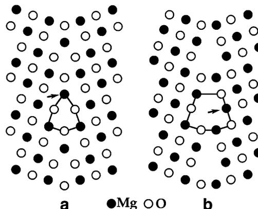
FIG. 3. Grain boundary structure models for a  $\Sigma = 5$  {310}  $\langle 001 \rangle$  tilt boundary in NaCl-type ceramics (a) proposed by Kingery [16] (b) calculated by Duffy and Tasker [11], and Harris *et al.* [9] for NiO and MgO, respectively. The site with the largest calcium segregation energy for both structures is indicated with a black arrow.
