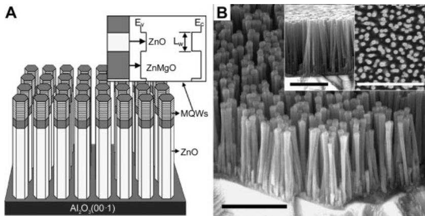
Fig. 1. A) Schematic of multiple quantum well (MQW) nanorods consisting of 10 periods of  $\text{Zn}_{0.8}\text{Mg}_{0.2}\text{O}/\text{ZnO}$  on the tips of ZnO nanorods. An electronic band diagram for the MQW is inset. B) FE-SEM images of the MQW nanorods. Scale bar: 0.5  $\mu\text{m}$ .
