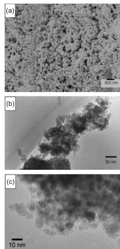
Fig. 1. The SEM and TEM images of a Ni:PVA film heat-treated at 923 K: a) SEM image, b) low-magnification TEM image, and c) high-magnification TEM image.
